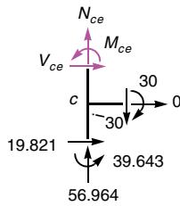
$$\begin{aligned}\sum M &= 0: M_{ce} - 30 - 39.643 = 0 \Rightarrow M_{ce} = -69.643 \\ \sum V &= 0: -N_{ce} + 30 - 56.964 = 0 \Rightarrow N_{ce} = -26.964 \\ \sum H &= 0: V_{ce} + 19.821 = 0 \Rightarrow V_{ce} = -19.821\end{aligned}$$
