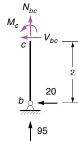
$$\begin{aligned}\sum M_{(c)} = 0: \quad -20 \cdot 2 + M_{bc} &= 0 \Rightarrow M_{bc} = 40 \\ \sum V = 0: \quad -95 - N_{bc} &= 0 \Rightarrow N_{bc} = -95 \\ \sum H = 0: \quad -20 - V_{bc} &= 0 \Rightarrow V_{bc} = -20\end{aligned}$$
