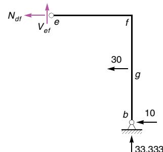
$$\sum V = 0: -V_{ef} - 33.333 = 0 \Rightarrow V_{ef} = -33.333$$
