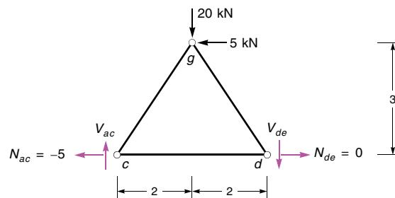
$$\begin{aligned}\sum M_{(c)} &= 0: 5 \cdot 3 - 20 \cdot 2 - V_{de} \cdot 4 = 0 \Rightarrow V_{de} = -6.25 \\ \sum V &= 0: 20 - 6.25 - V_{ac} = 0 \Rightarrow V_{ac} = 13.75\end{aligned}$$
