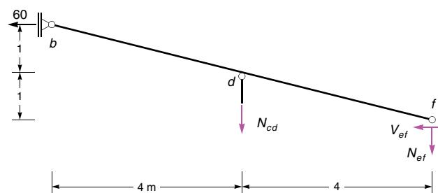
$$\begin{aligned}\sum M_{(f)} &= 0: N_{cd} \cdot 4 + 60 \cdot 2 = 0 \Rightarrow N_{cd} = -30 \\ \sum V &= 0: N_{ef} - 30 = 0 \Rightarrow N_{ef} = 30 \\ \sum H &= 0: -V_{ef} - 60 = 0 \Rightarrow V_{ef} = -60\end{aligned}$$
