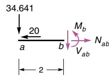
$$\begin{aligned} \sum M_{(b)} = 0: 34.641 \cdot 2 + M_b = 0 \Rightarrow M_b = -69.282 \\ \sum V = 0: 34.641 + V_{ab} = 0 \Rightarrow V_{ab} = -34.641 \\ \sum H = 0: -20 + N_{ab} = 0 \Rightarrow N_{ab} = 20 \end{aligned}$$
