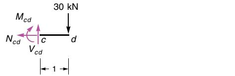
$$\begin{aligned}\sum M(c) &= 0: -M_{cd} - 30 \cdot 1 = 0 \Rightarrow M_{cd} = -30 \\ \sum V &= 0: -V_{cd} + 30 = 0 \Rightarrow V_{cd} = 30 \\ \sum H &= 0: N_{cd} = 0\end{aligned}$$
