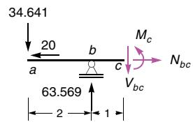
$$\begin{aligned} \sum M_{(c)} = 0: 34.641 \cdot 3 - 63.569 \cdot 1 + M_c = 0 \Rightarrow M_c = -40.354 \\ \sum V = 0: 34.641 - 63.569 + V_{ab} = 0 \Rightarrow V_{ab} = 28.928 \\ \sum H = 0: -20 + N_{ab} = 0 \Rightarrow N_{ab} = 20 \end{aligned}$$
