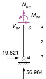
$$\begin{aligned}\sum M(c) &= 0: M_{ca} + 19.821 \cdot 2 = 0 \Rightarrow M_{ca} = 39.643 \\ \sum V &= 0: -N_{ac} - 56.964 = 0 \Rightarrow N_{ac} = -56.964 \\ \sum H &= 0: V_{ac} + 19.821 = 0 \Rightarrow V_{ac} = -19.821\end{aligned}$$
