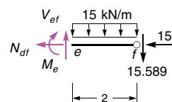
$$\begin{aligned}\sum M(e) &= 0: -15 \cdot 2^2 / 2 - 15.589 \cdot 2 - M_e = 0 \Rightarrow M_e = -61.178 \\ \sum V &= 0: 15 \cdot 2 + 15.589 - V_{ef} = 0 \Rightarrow V_{ef} = 45.589 \\ \sum H &= 0: -15 - N_{df} = 0 \Rightarrow N_{df} = -15\end{aligned}$$
