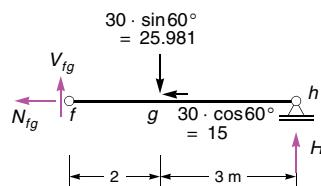
$$\begin{aligned}\sum M(f) &= 0: -25.981 \cdot 2 + H \cdot 5 = 0 \Rightarrow H = 10.392 \\ \sum V &= 0: -10.392 + 25.981 - V_{fg} = 0 \Rightarrow V_{fg} = 15.589 \\ \sum N &= 0: -15 - N_{fg} = 0 \Rightarrow N_{fg} = -15\end{aligned}$$
