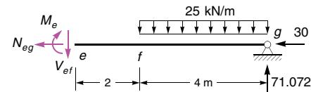
$$\begin{aligned} \sum M_{(e)} = 0: 71.072 \cdot 6 - 25 \cdot 4 \cdot 4 - M_e = 0 \Rightarrow M_e = 26.432 \\ \sum V = 0: -71.072 + 25 \cdot 4 + V_{ef} = 0 \Rightarrow V_{ef} = -28.928 \\ \sum H = 0: -30 - N_{eg} = 0 \Rightarrow N_{eg} = -30 \end{aligned}$$
