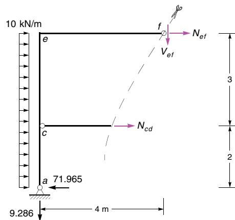
$$\sum V = 0: 9.286 + V_{ef} = 0 \Rightarrow V_{ef} = -9.286$$
