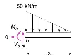
$$\begin{aligned}\sum M_{(b)} &= 0: -M_b - 50 \cdot 3/2 \cdot 1 = 0 \Rightarrow M_c = -75 \\ \sum V &= 0: -V_{b,\text{re}} + 50 \cdot 3/2 = 0 \Rightarrow V_{b,\text{re}} = 75\end{aligned}$$
