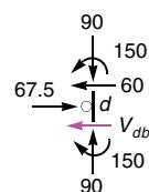
$$\sum H = 0: 67.5 - 60 - V_{db} = 0 \Rightarrow V_{db} = 7.6$$
