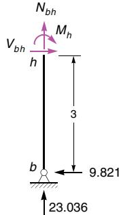
$$\begin{aligned}\sum M(h) &= 0: -M_h - 9.821 \cdot 3 = 0 \Rightarrow M_e = -29.464 \\ \sum V &= 0: -N_{bh} - 23.036 = 0 \Rightarrow N_{bh} = -23.036 \\ \sum H &= 0: V_{bh} - 9.821 = 0 \Rightarrow V_{bh} = 9.821\end{aligned}$$
