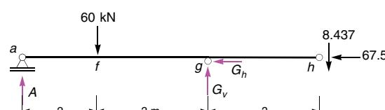
$$\begin{aligned}\sum M_{(a)} = 0: \quad & -60 \cdot 2 - 8.437 \cdot 8 + G_v \cdot 5 = 0 \Rightarrow G_v = 37.5 \\ \sum V = 0: \quad & 60 - 37.5 + 8.437 - A = 0 \Rightarrow A = 30.937 \\ \sum H = 0: \quad & 67.5 - G_h = 0 \Rightarrow G_h = -67.5\end{aligned}$$
