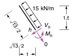
$$\begin{aligned}\sum M_{(h)} = 0: \quad & 15 \cdot (\sqrt{13}/2)^2 / 2 + M_h = 0 \Rightarrow M_h = -24.375 \\ \sum F_{\perp} = 0: \quad & 15 \cdot \sqrt{13}/2 + V_{h,o} = 0 \Rightarrow V_{h,o} = -27.042\end{aligned}$$
