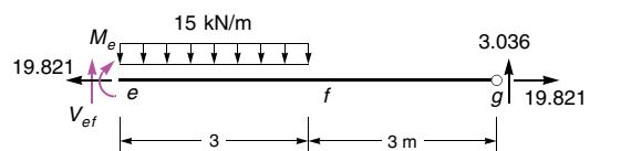
$$\begin{aligned}\sum M(e) &= 0: -M_e - 15 \cdot 3^2 / 2 + 3.036 \cdot 6 = 0 \Rightarrow M_e = -49.286 \\ \sum V &= 0: -V_{ef} + 15 \cdot 3 - 3.036 = 0 \Rightarrow V_{ef} = 41.964\end{aligned}$$
